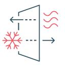
With FINEO insulating glass you will feel much warmer compared to single or double glazing. Why? Due to FINEO's exceptional low u-value, the internal pane is warmer, which in turn eliminates draughts and cold spots.
